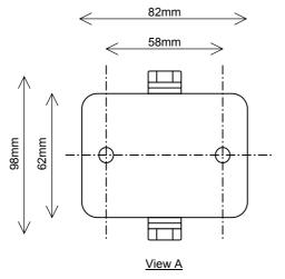
2off - Fixing holes 6.25mm (0.25") Dia.
